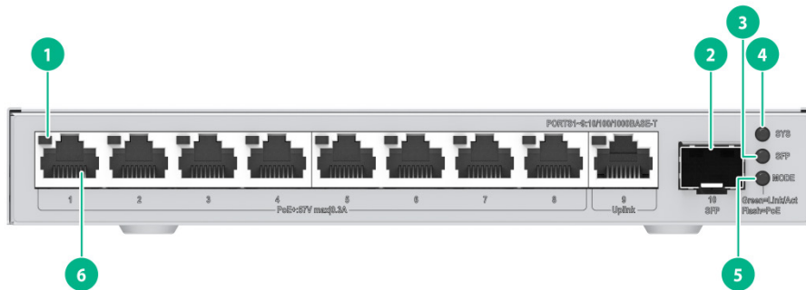
Figure 7 Front Panel Diagram of S1600V2-10P-HPWR
